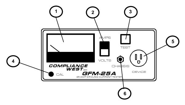
Figure 2-1. Controls, Indicators, Connectors – Example Model GFM-40ac Front Panel
