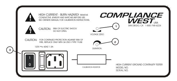
Figure 2-2. Controls, Indicators, Connectors - Model GFM-40ac Rear Panel
